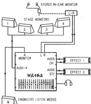
**Studio or Location Recording -** Multitracking up to 16tracks with stereo mastering and recording. Stereo cue for the performers, and plenty of effects.
