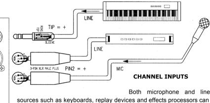
be plugged into either the jack or XLR input for convenience. The channel accepts a wide 70dB range of source levels. The input is a balanced 3-wire to provide the best immunity to interference pickup on long cable runs. However, you can plug in an unbalanced 2-wire source simply by linking the input - (cold) connection to ground (XLR pin3 to pin 1, jack ring to sleeve) in the connector plug.
