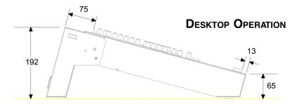
The console is fitted with rubber feet to ensure it does not slip or scratch the work surface. The control panel is angled at 15 degrees for operating convenience.
