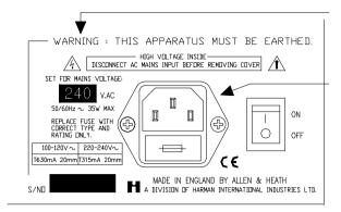
Refer to the **SAFETY WARNING** on page 3 of this User Guide. Check that the voltage indicated on the rear panel is the same as the mains supply in your area. Check that the correct mains lead with moulded plug has been supplied with your console. Read and understand the warnings and instructions printed on the rear panel and shown here.
