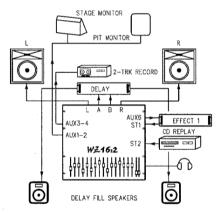
**Houses of Worship** - Increasingly sophisticated sound control is required. Here, a music PA is controlled using L-R, and the congregation PA with delay compensation separately controlled using A-B.
