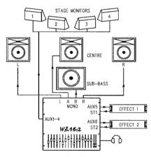
**Dedicated Stage Monitor -** This example shows 4 floor wedges for the musicians and a stereo in-ear monitor for the lead performer. The engineer monitors the signals using a floor wedge similar to the stage monitors.
