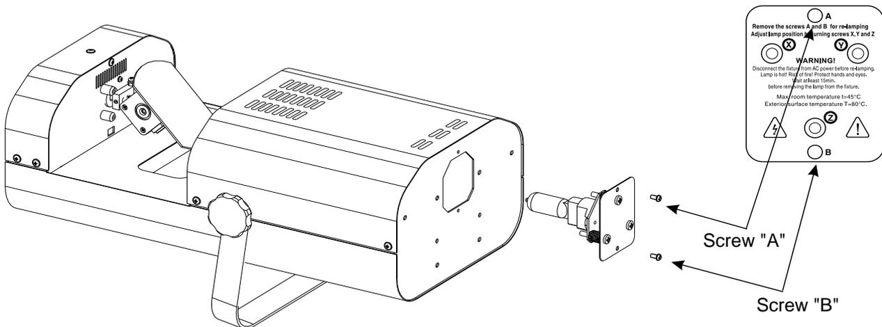
To insert the lamp (MSD 250 or MSD 250/2) open the small cover at the rear panel (see the drawing) by loosening the 2 Phillips screws "A" and "B" on the cover.
