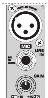
Fig. 2.1: Connectors and controls of mic/line inputs
